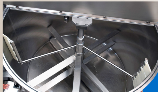
shown: slurry scraper and blades
